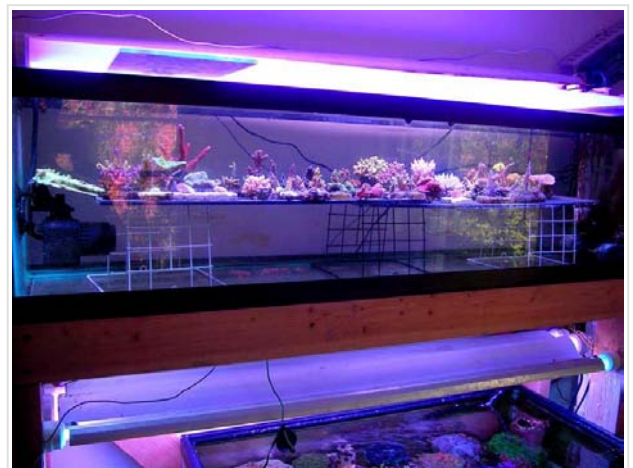
Figure 2 This horizontal gyre tank produced flow speeds between 15-22cm/s.
